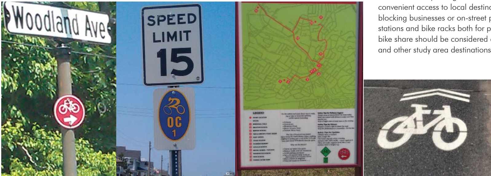
Bike routes should be clearly marked both on the roadway pavement and with wayfinding signage and route markers.
