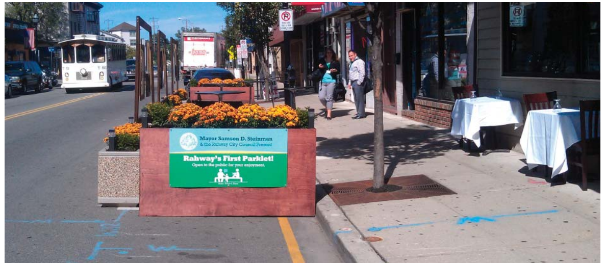
Parklets are raised platforms flush with the sidewalk that extend into one to three parallel parking spaces and can be effective ways to test traffic calming on a temporary basis.
