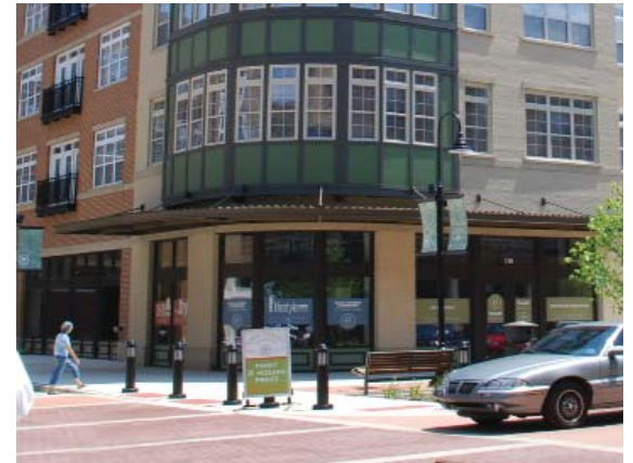
Textured paved intersections with protective bollards help to calm traffic speeds, raise awareness of pedestrian activity and landmark downtown areas
